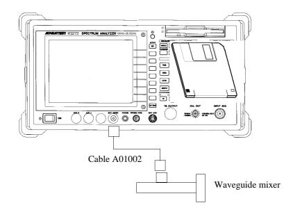
Figure 2-1 Cable Connection between the R3273 and Waveguide Mixer
